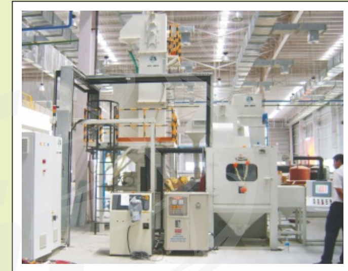
CNC Robotic Shot Peening Machine For Titanium Alloy Beam
