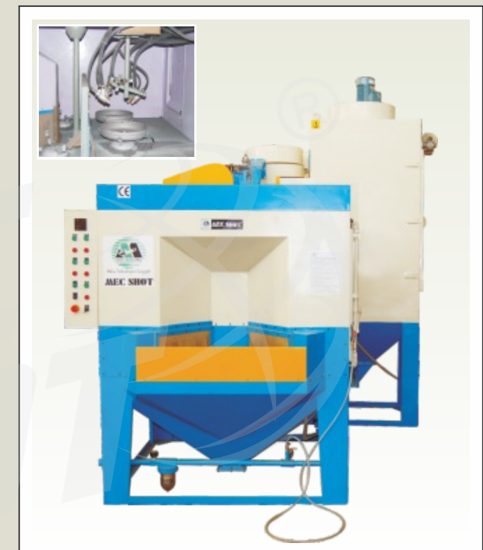
Suction Blasting Machine with Indexing Turn Table Model SB-SP4 for Cookware Industry
