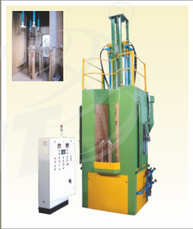
Shot Blasting Machine for removing scale and rounding of sharp corner of fluted roller for textile machinery. Features with six rotating satellites mounted on indexing turntable with vertical gun reciprocation.
