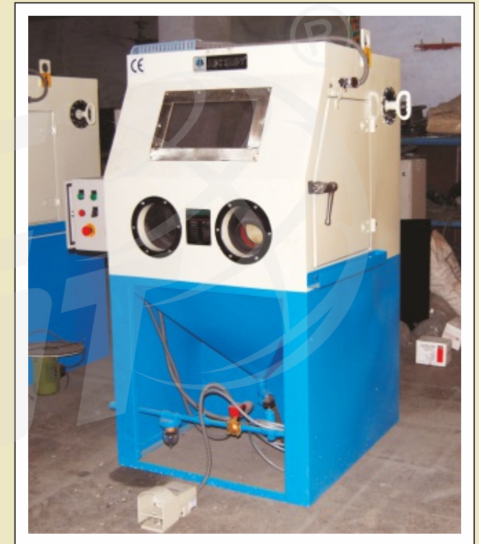
MEC SHOT Compact Super Blasting Machine with Reclaimer & Dust Collector
