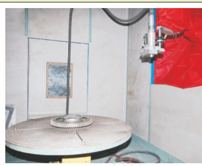
CNC Robotic Shot Peening Machine For Gas Turbine Blades
