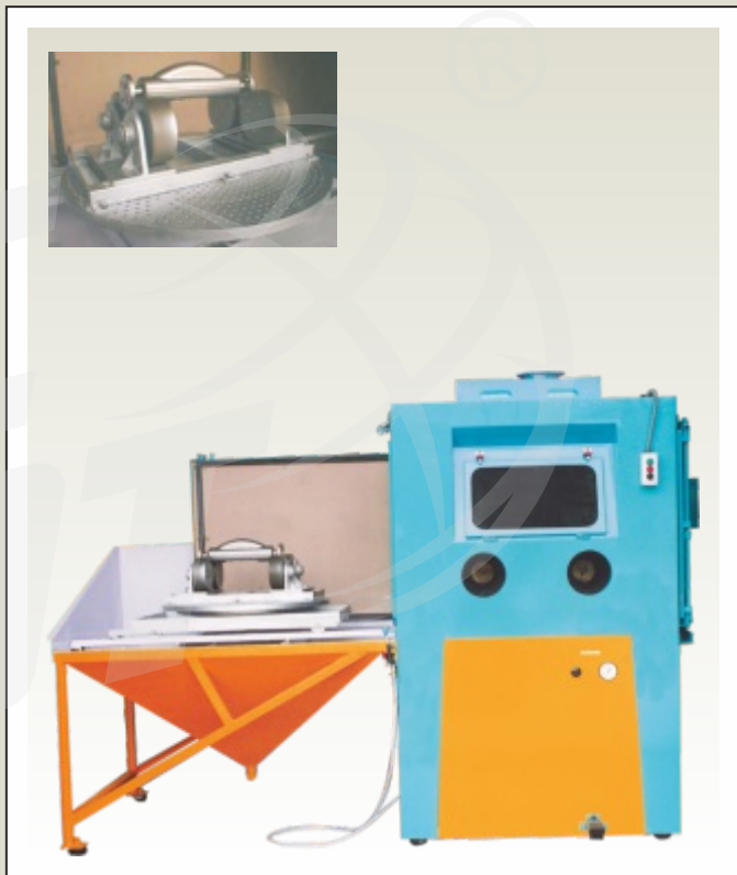
Special Purpose Glass Bead Blasting Machine for Flow Meter (Promass Sensor) featured with inside turn table and track extension, job holding fixture and ultra wired cartridge type micro filters for most efficient dust collection.
