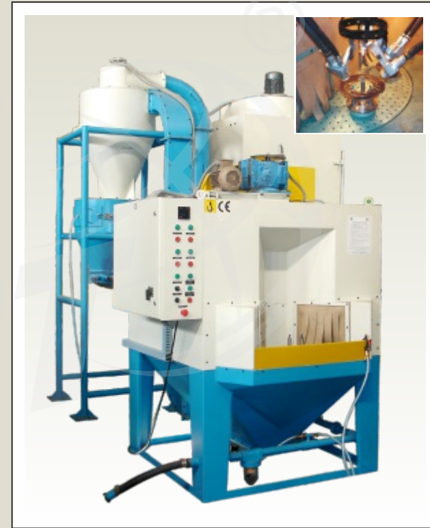
Suction Abrasive Blasting Cabinet to blast clean the inside holes & outer periphery of disc brake. Pleated bag dust collector is provided for very low dust emission level.
