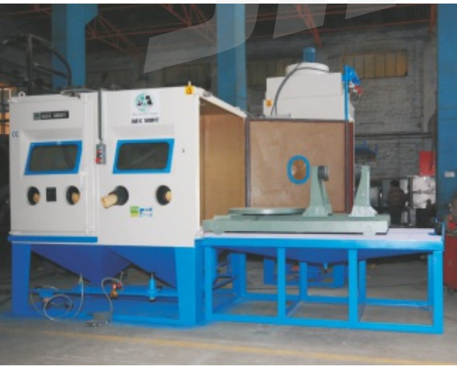
Abrasive Blasting Cabinet Super Blaster to Blast Clean Stainless Steel Turbo Charger Components
