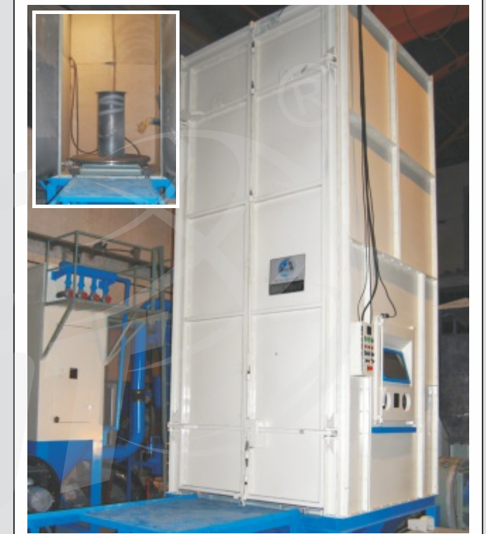
Special Suction Blaster with Track Extension & Turn Table for Refinery Jobs
