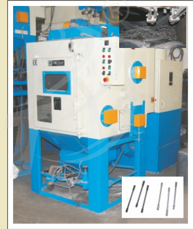
Belt Tumbler Type Abrasive Blasting Machine for Steering Mechanism of Automobile Industry
