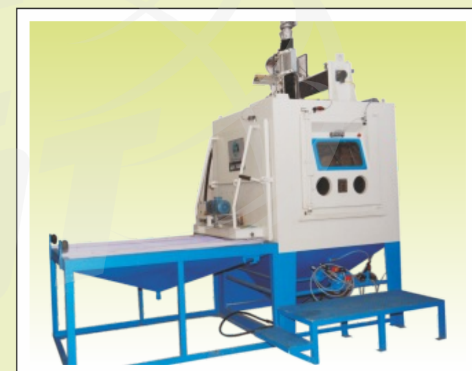
Wet Ceramic Beads Shot Peening Machine for Aero engine Parts
