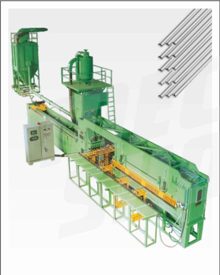
Automatic Blast Cleaning of Zirconium Tubes. Five tubes of max. 10 mtrs. Long are cleaned internally at a time in about 3 minutes.
