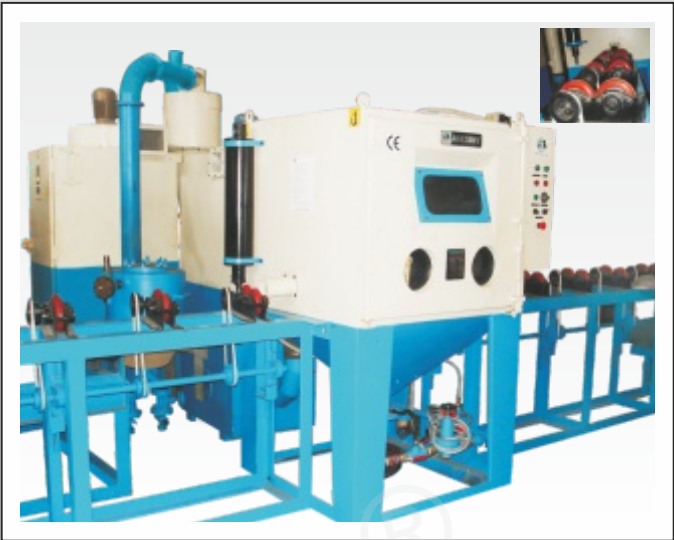
Automatic Blasting Machine for External Cleaning of Metallic Rods / Pipes
