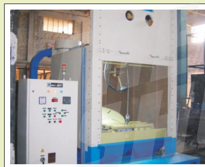
Dry Shot Peening Machine For Aviation Components
