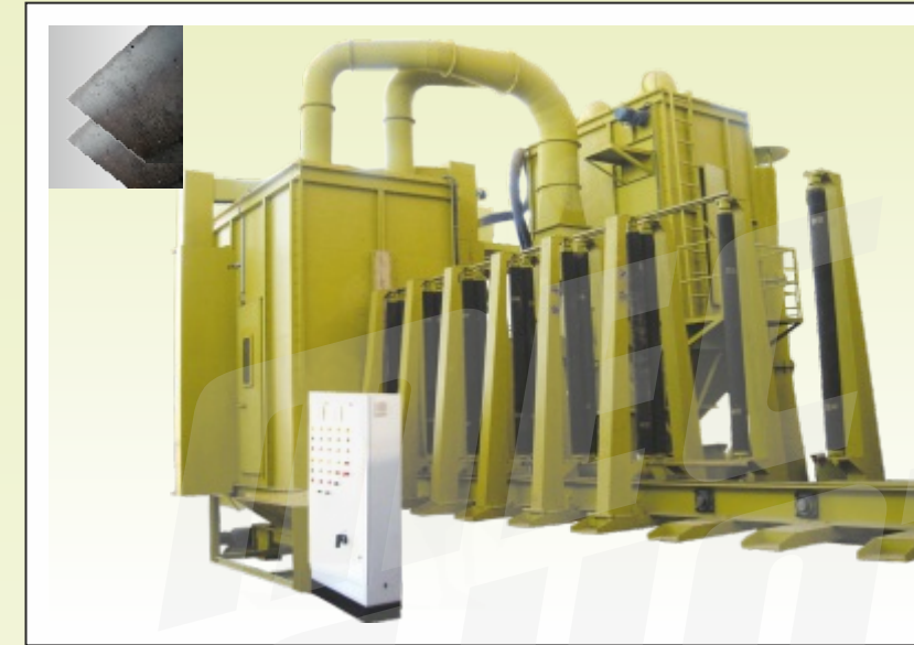
Plate Cleaning Machine featured with vertical sheet movement through motorised roller conveyor and blast nozzle reciprocation through chain sprocket & AC variable drive.
