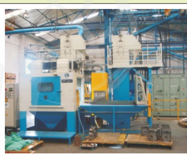
Shot Peening Machine For Cylinder Blocks
