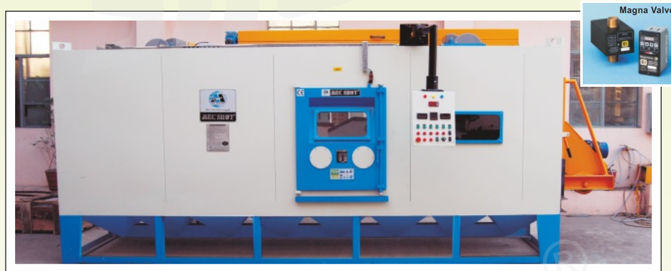
Automatic Machine for Etching Rollers used in steel strips rolling mills. Blast Nozzles reciprocate horizontally while roller rotates at preset speed with additional features like: Magna Valve for Abrasive Flow Control and Support Arm Control Panel
