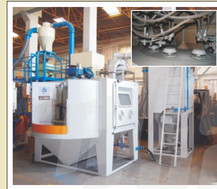
Automatic Continuous Blasting Machine for Brake Shoes featured with slow RPM turntable, concave reciprocation of nozzles.
