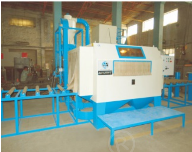
Special Pressure Blasting Machine with X-Y Manipulator & Internal Cleaning Lance Nozzle For Submersible Pump Casing
