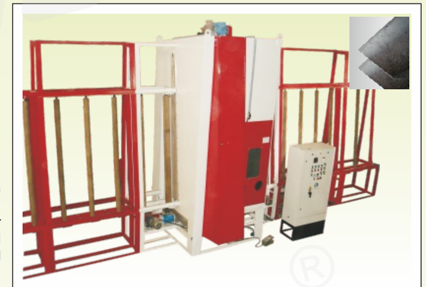
Blast Cabinet for etching on Stainless Steel Sheet. Featured with inclined roller arrangement for support and movement of Stainless Steel Sheet.
