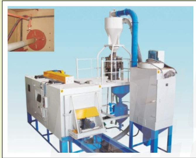
Automatic Machine for Etching Rollers used in steel strips rolling mills. Blast Nozzles reciprocate horizontally while roller rotates at preset speed
