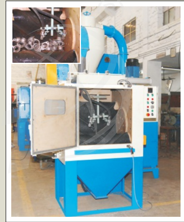
Belt Tumbler Type Shot Blasting Machine for Cleaning of Anti Vibrating Pads for Automobiles Industries
