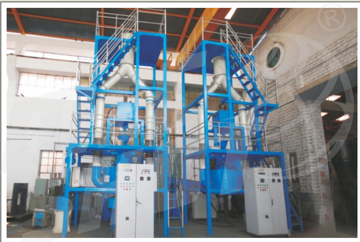
"MEC SHOT" Special Sand Blast Cleaning M/c For Locomotive Wheels After Moulding In Hot Condition Before Machining.
