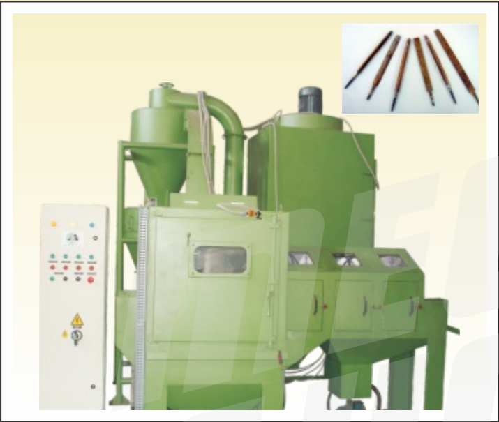
Mec Shot semi-automatic blasting machine for surface preparation of files (hand tool)
